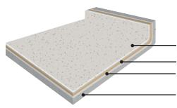
ISO-103 Topcoat EPO-204 Grout Coat PUR-Guard HD-SL with RT-Sand Concrete
