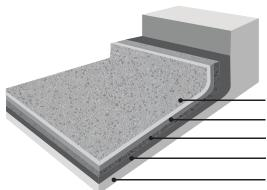
EPO-204 Topcoat EPO-204 Grout Coat Colored Quartz PUR-Guard HD-SL Concrete
