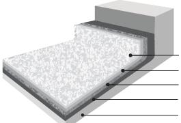
EPO-204 Topcoat EPO-204 Grout Coat Colored Flake PUR-Guard HD-SLE Concrete
