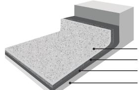
ISO-101 Topcoat Colored Quartz PUR-Guard HD-SL Concrete
